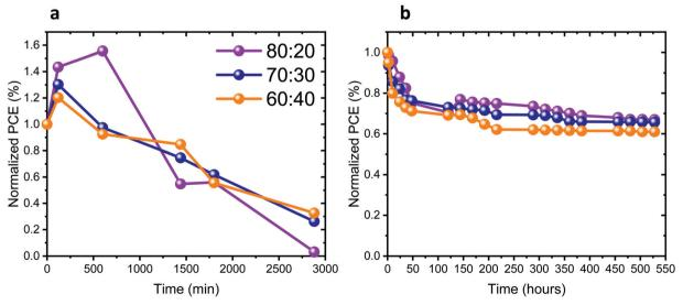
Fig. 7 (a) Stability under 1 sun illumination of complete solar cells with different ratios of Pb: Sn as discussed in this work. (b) Stability of the cells stored under an inert atmosphere and measured in the open air with encapsulation.
