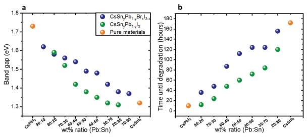
Fig. 2 (a) The band gap as a function of the Pb: Sn ratio for the cases of mixed iodide and bromide and for pure iodide compounds. The slope of the green dots is 1.5 times larger than the slope of the blue dots. (b) Photostability measurements under 1 sun illumination, 18 °C and 27% humidity. The data in this graph are based on the absorbance spectra shown in Fig. S4 and S5 (ESI†).
