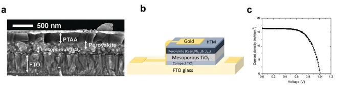
Fig. 6 (a) Cross section SEM image of the PSC with a ratio of 80: 20 (CsSn<sub>0.2</sub>Pb<sub>0.8</sub>I<sub>2.6</sub>Br<sub>0.4</sub>) (Pb: Sn) and PTAA as the HTM. (b) Schematic illustration of the perovskite solar cell configuration used in this work. (c) JV curve of the champion cell presenting 12.7% efficiency, a FF of 64.2%, a  $J_{sc}$  of 19.09 mA cm<sup>-2</sup> and a  $V_{oc}$  of 1 V.
