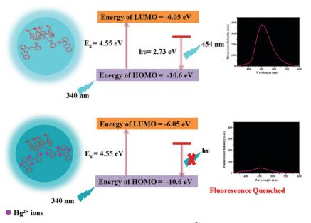
Scheme 2 Schematic representation of the plausible mechanism for the binding of  $Hg^{2+}$  ions with the as-synthesized CDs.
