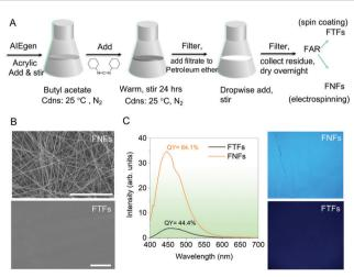
Fig. 1 Physical and optical properties of FNFs and FTFs. (A) A generalized scheme for the synthesis of FNFs and FTFs which involve first knitting the AlEgen to the acrylic polymer. (B) SEM images of the materials (scale bar is 50  $\mu$ m). (C) Fluorescence spectra captured from the FTFs and FNFs together with their QY numbers and UV light (365 nm) images
