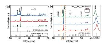
Fig. 1 (a) Powder XRD patterns for  $Na_{0.03}Sn_{0.97}Se-5\%$ Te in different processes; (b) bulk XRD patterns for  $Na_{0.03}Sn_{0.97}Se-x\%Te$  (x = 0, 5 and 15) measured on the surface perpendicular to the pressing direction.
