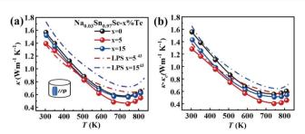
Fig. 4 Temperature dependences of (a) thermal conductivity; (b) lattice thermal conductivity. The data for the LPS samples are plotted for comparison.43
