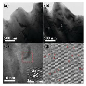
Fig. 5 Microstructure of the LPHD samples: (a) low-magnification TEM image of Na<sub>0.03</sub>Sn<sub>0.97</sub>Se-0%Te; (b) low-magnification TEM image of  $Na_{0.03}Sn_{0.97}Se-5\%$ Te with the defects in the matrix; (c) HRTEM image from (b) the region marked 1 with the FFT image and its interplanar spacing; (d) inverse FFT image of the red box in panel (c) obtained from the (400) reflection.
