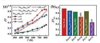
Fig. 6 (a) Temperature dependence of ZT for LPHD samples; (b) average ZT values from 300 to 810 K for our Na<sub>0.03</sub>Sn<sub>0.97</sub>Se-5%Te LPHD sample and other previously reported polycrystalline  $Na_{0.03}Sn_{0.97}Se$  samples.  $^{31,32,43,44,60}$
