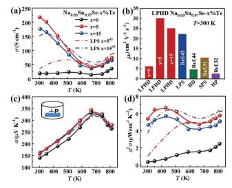
Fig. 3 Temperature dependence of  $Na_{0.03}Sn_{0.97}Se-x\%Te$  (x = 0, 5 and 15) samples: (a) electrical conductivity, (b) room temperature Hall mobility with some previous reports as a comparison, (c) Seebeck coefficient and (d) power factor
