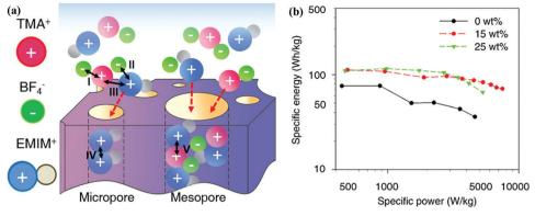
Fig. 13 Schematic of the selective charging behavior of  $TMABF_4/EMIMBF_4$  ionic mixture electrolyte (a). Ragone plots (b). (Reproduced with permission. <sup>203</sup> Copyright 2017, American Chemical Society.)
