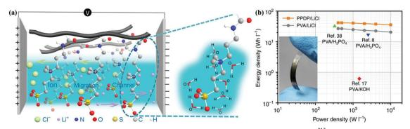
Fig. 14 Zwitterionic PPDP under an external electric field (a). Ragone plots (b). (Reproduced with permission.<sup>213</sup> Copyright 2016, Springer Nature.)
