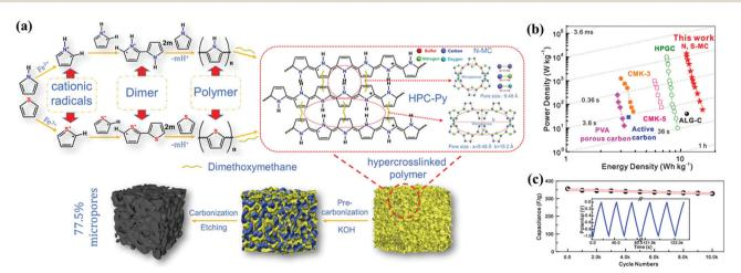
Fig. 6 Synthesis of hypercrosslinked polymer-derived carbons (a). Ragone plots (b). Long-term cycling performance (c). (Reproduced with permission.<sup>78</sup> Copyright 2019, Elsevier.)
