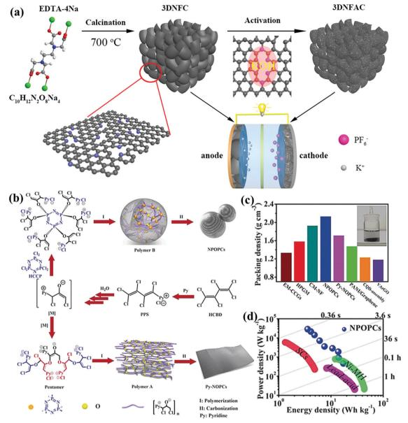
Fig. 9 Schematic illustration of N-rich 3D hierarchical porous carbons (a). (Reproduced with permission. 127 Copyright 2019, Elsevier.) Synthesis of multiheteroatom-doped porous carbons (b). Packing density (c). Ragone plots (d). (Reproduced with permission 133 Copyright 2019, Wiley-VCH.)
