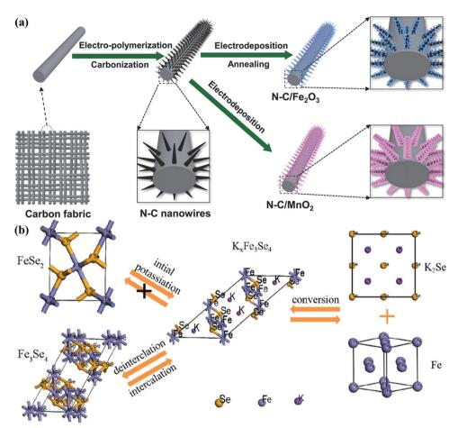
Fig. 10 Schematic of N-doped carbon nanowires@MnO<sub>2</sub> and N-doped carbon nanowires@Fe<sub>2</sub>O<sub>3</sub> (a). (Reproduced with permission.  $^{147}$  Copyright 2018, Wiley-VCH.) Schematic for the potassium storage reaction mechanism (b). (Reproduced with permission.  $^{157}$  Copyright 2019, Wiley-VCH.)
