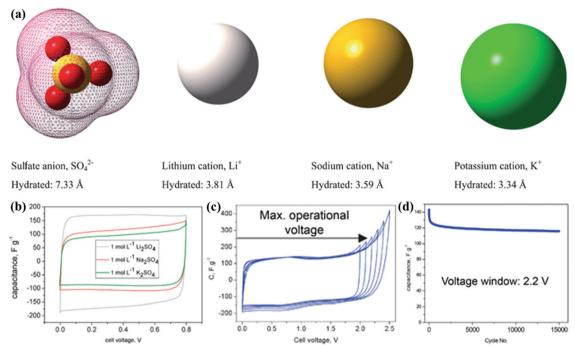
Fig. 11 Ion shapes/dimensions in aqueous solutions (a). Cyclic voltammograms in 1 mol  $L^{-1}$  Li<sub>2</sub>SO<sub>4</sub>/Na<sub>2</sub>SO<sub>4</sub>/Ka<sub>2</sub>SO<sub>4</sub> at 1 mV s<sup>-1</sup> (b) and 1 mol  $L^{-1}$  Li<sub>2</sub>SO<sub>4</sub> at 10 mV s<sup>-1</sup> (c). Cyclability in 1 mol L<sup>-1</sup> Li<sub>2</sub>SO<sub>4</sub> under 2.2 V (d). (Reproduced with permission. 162 Copyright 2012, The Royal Society of Chemistry.)
