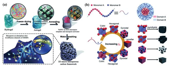
Fig. 8 Schematic illustration of the synthesis of hierarchical porous carbons from a gelatin-NaNO<sub>3</sub> biopolymer (a). (Reproduced with permission. 104 Copyright 2018, Wiley-VCH.) Examples of porous carbon structures after the calcination of block copolymers (b). (Reproduced with permission.<sup>92</sup> Copyright 2019, The Royal Society of Chemistry.)
