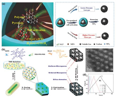
Fig. 7 Schematic illustration of monodispersed mesoporous carbon spheres (a). (Reproduced with permission.<sup>85</sup> Copyright 2018, Wiley-VCH.) Schematic illustration of ordered mesoporous carbons (b). TEM image (c). Galvanostatic charge/discharge curves (d). (Reproduced with permission.98 Copyright 2016, Elsevier.)
