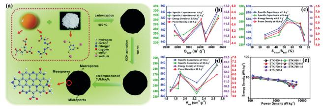
Fig. 2 Schematic of the preparation of egg yolk-derived activated carbons (a). Influence among the structural parameters, i.e., S<sub>BET</sub> (b); S<sub>micro</sub>/S<sub>BET</sub> (c);  $V_{\mathrm{tot}}$  (d); and electrochemical performances such as specific capacitance, power density, energy density, and rate density. Ragone plots (e). (Reproduced with permission.<sup>30</sup> Copyright 2018, The Royal Society of Chemistry.)
