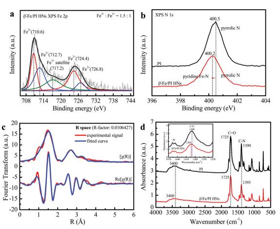
Fig. 3 Local chemical environment and fine structure of surface elements. (a) Fe 2p XPS spectrum of If-Fe/PI HNs. (b) N 1s XPS spectra of PI and If-Fe/PI HNs. (c) Fe K-edge EXAFS oscillation and its curve fitting of If-Fe/PI HNs. (d) FTIR spectra of PI and If-Fe/PI HNs.
