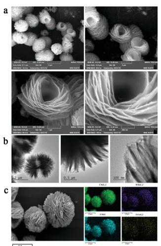
Fig. 2 Morphology and structure of If-Fe/PI HNs. (a) SEM images with different amplifications of If-Fe/PI HNs. (b) TEM images with different amplifications of If-Fe/PI HNs. (c) Corresponding SEM elemental mapping analysis for C, N, O and Fe of If-Fe/PI HNs.
