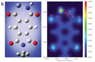
**Fig. 4** Non-uniform distribution of surface electrons on lf-Fe/PI HNs. (a) EPR spectra of PI and lf-Fe/PI HNs. (b) DFT calculations for the optimized structure of lf-Fe/PI HNs in one unit (left) and the corresponding two-dimensional valence-electron density color-filled maps of the lf-Fe/PI HNs model (right). Purple, red, grey and blue circles denote Fe, O, C and N atoms, respectively. The valence-electron density is given in e Å<sup>-3</sup>.
