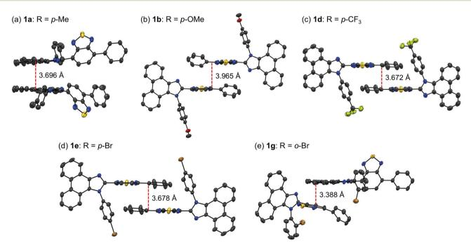
Fig. 5 Molecular structures with an adjacent molecule of 1a, 1b, 1d, 1e and 1g with thermal ellipsoids at 50% probability. All hydrogen atoms are omitted for clarity. Color code: gray = C; blue = N; red = O; green = F; yellow = S; and orange = Br.
