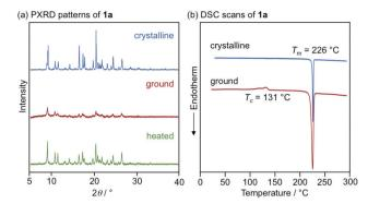
Fig. 8 (a) PXRD patterns for the powdered crystalline (blue), ground (red), and heated (green) samples of 1a. (b) DSC scans for crystalline (blue) and ground (red) samples of **1a**.  $T_m$  and  $T_c$  values are noted near the corresponding peaks.
