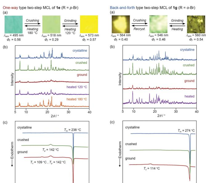
**Fig. 9** (a) Photographs for the two-step MCL of **1e** excited with UV light (365 nm). (b) PXRD patterns for the crystalline (blue), crushed (green), ground (red), and heated (120 °C, purple and 180 °C, orange) samples of **1e**. (c) DSC scans for the crystalline (blue), crushed (green), and ground (red) samples of **1e**.  $T_{\rm m}$ ,  $T_{\rm p}$ , and  $T_{\rm c}$  values are noted near the corresponding peaks.
