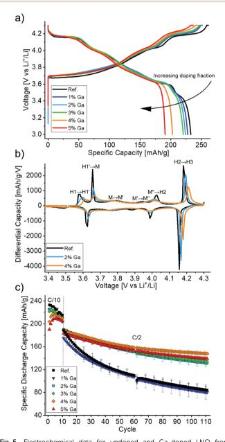
Fig. 5 Electrochemical data for undoped and Ga-doped LNO from galvanostatic cycling of half-cells at 25 °C in the voltage range between 3.0 and 4.3 V vs. Li<sup>+</sup>/Li. (a) 1st cycle voltage profiles. (b) 3rd cycle differential capacity plots. Only selected samples are shown for clarity. (c) Specific discharge capacity over 110 cycles.
