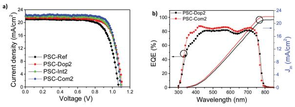
Fig. 5 J-V characteristics at 1 sun illumination of each engineering approach and the EQE spectrum of a representative device. (a) J-V curves of PSC-Ref (black), PSC-Dop2 (red), PSC-Int2 (green), and PSC-Com2 (blue). (b) Representative EQE of PSC-Int2 and PSC-Com2. The integrated current density of the device's spectral response with the AM1.5G photon flux spectrum is depicted on the right axis.
