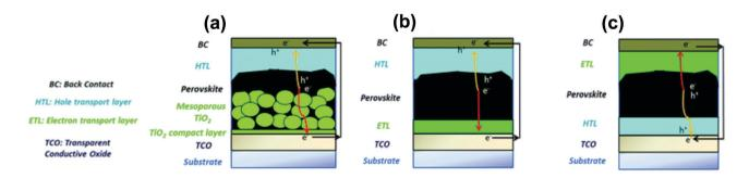
Fig. 1 Perovskite solar cell architectures: (a) n-type TiO<sub>2</sub> mesoporous-based; (b) planar "n-i-p"; (c) planar "p-i-n". Illumination occurs from the substrate side. In all these cases, the substrate can be either a glass or polymer foil. Reproduced with permission from ref. 48. Copyright © 2017 The Royal Society of Chemistry
