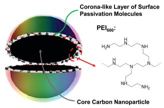
Fig. 1 A cartoon illustration on the structure in CDots in general and PEI<sub>600</sub>-CDots specifically.
