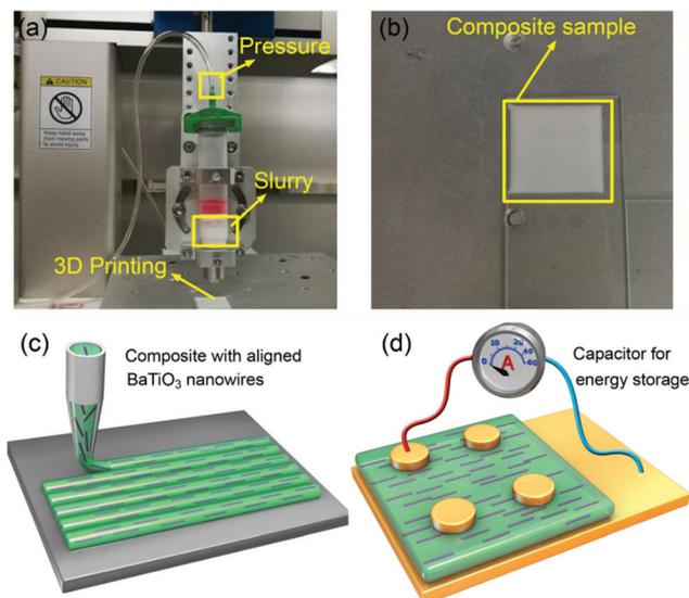
Fig. 1 Alignment of BaTiO<sub>3</sub> nanowires in nanocomposites: photographs of (a) the printing assembly and (b) a printed nanocomposite sample; schematic illustrations of (c) the alignment of BaTiO<sub>3</sub> nanowires in the P(VDF-CTFE) matrix and (d) a nanocomposite capacitor for energy storage applications.
