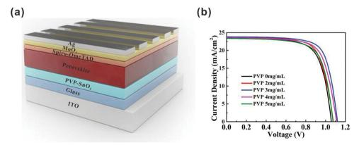
Fig. 1 (a) Schematic view of the device structure in this work. (b) J-V characteristics of PSCs with PVP-SnO<sub>2</sub> ETLs with various amounts of PVP.
