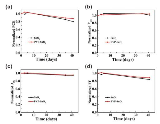
Fig. 6 The shelf-stability of perovskite solar cells in a glove box without any encapsulation. Normalized (a) PCE, (b)  $V_{\rm OC}$ , (c)  $J_{\rm SC}$  and (d) FF.
