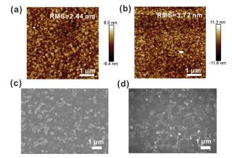
Fig. 3 AFM images of the SnO<sub>2</sub> (a) and the PVP-SnO<sub>2</sub> (b) films deposited on ITO. SEM images of the perovskites coated on the SnO<sub>2</sub> film (c) and the PVP-SnO<sub>2</sub> film (d)
