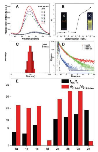
Fig. 4 (A) Fluorescence spectra of 2b in DMSO/water with different water fractions. (B) The  $I/I_0$  ratios of **2b** in DMSO/water with different water fractions. (C) Particle size distribution of **2b** in a DMSO/water mixture with an  $f_P$  value of 99%. (D) Emission decay of 2b in DMSO, H2O, and the solid state. (E) Ratio of the quantum yields for the solid and solution states of all compounds, and the ratio of the fluorescence intensity in the aggregation and solution states.
