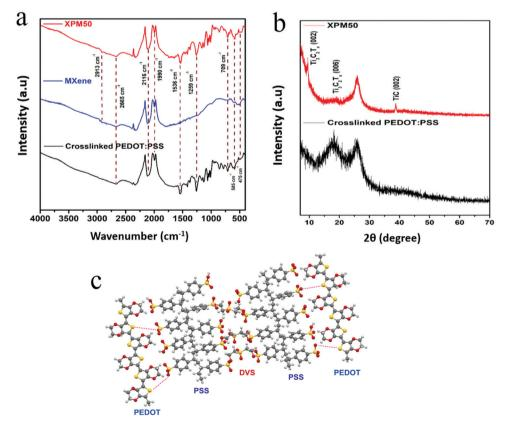
Fig. 3 (a) Comparison of the FTIR spectra of XPM50, the MXene and crosslinked PEDOT:PSS. (b) Comparison of the powder XRD patterns of XPM50 and crosslinked PEDOT:PSS. (c) Crosslinking mechanism.
