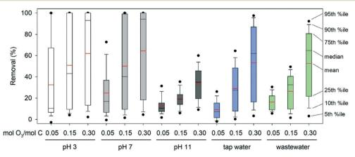
Fig. 3 Box and whisker plots of the removal of the 90 OMPs under the different conditions used in this study. %ile: percentile.
