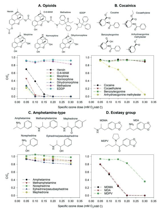
Fig. 2 Abatement of illicit drugs and their metabolites as a function of the specific ozone dose in pure buffered water at pH 7. All compounds were added as a mixture of 90 OMPs in total. Error bars from duplicate analysis of samples were omitted for figure overview and are provided in the ESI† xlsx-data file
