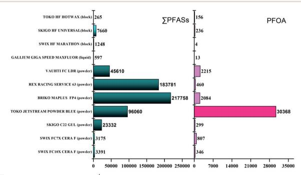
Fig. 1  $\sum$ PFAS and PFOA concentrations (ng g<sup>-1</sup>) in the eleven commercial ski wax products purchased from a Norwegian retailer in 2019. Concentrations exceeding the highest calibration point are marked with darker colours.
