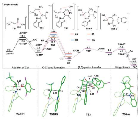
Fig. 1 The relative Gibbs free energy profiles of the isothiourea-catalyzed [3 + 3] annulation reaction. (the superscript "3" represents adding the free energy of pre-R2, the superscript "b" represents the S configuration, and distances are in angstroms).
