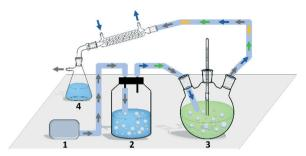
Fig. 2 A schematic diagram of the TBCR system (not proportionally scaled). Area 1 is a pump unit. Area 2 is a buffer unit containing 2-propanol and water. Area 3 is a reaction unit, in which the temperature is set at 30 °C. Area 4 is a collection unit. Air, water, 2-propanol and acetone are shown as gray, blue, green and yellow arrows, respectively. Air paths are shown as light blue lines.
