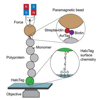
Fig. 3 Schematic diagram showing the key elements required to perform a single-molecule magnetic tweezers (MT) experiment.
