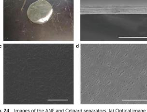
Fig. 24 Images of the ANF and Celgard separators. (a) Optical image of a neat aramid nanofiber (ANF) separator; (b) cross-sectional SEM image of a neat ANF separator; (c) SEM image of the surface of a neat ANF separator; (d) SEM image of the surface of Celgard 2325. Scale bars represent 30  $\mu m$ in (b), 500 nm in (c) and 3  $\mu m$  in (d). Reprinted with permission from ref. 398. (Creative Commons Attribution 4 International License.)
