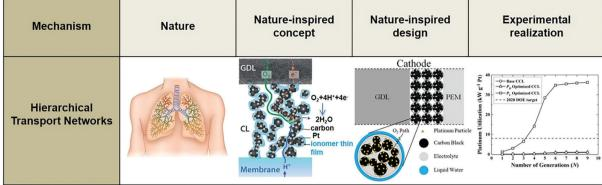
Fig. 17 Systematic methodology for the nature-inspired design of hierarchically structured electrocatalysts. Image of the porous catalyst layer structure ("Nature-inspired concept" section) was reproduced from ref. 350 with permission from the Royal Society of Chemistry
