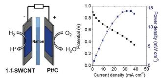
Fig. 11 Polarization (black) and power density (blue) curves for an MEA employing [Ni(P<sub>2</sub><sup>Cy</sup>N<sub>2</sub><sup>Arg</sup>)<sub>2</sub>]<sup>7+</sup> (denoted as 1-f-SWCNT) and Pt/C as the anode and cathode catalysts, respectively. Experimental conditions: anode loading: 0.3  $\mu g$  cm $^{-2}$ , cathode loading (Pt/C): 1 mg cm $^{-2}$ , Nafion $^{(\!R\!)}$  as the polymer electrolyte, 60 °C cell temperature. Reprinted with permission from ref. 297. Copyright 2017 Wiley-VCH.
