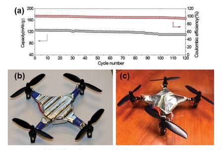
Fig. 23 (a) Cycling performance of the Zn/PZB-931/γ-MnO<sub>2</sub> battery at 0.2C; (b) and (c) two different designs of Zn/γ-MnO<sub>2</sub> battery pack as a replacement for the original device cover to supplement the main power source of unmanned aerial vehicles (UAVs). Reprinted with permission from ref. 397. Copyright 2019 American Chemical Society
