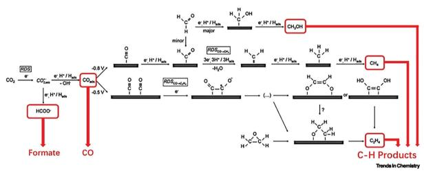
Fig. 15 Mechanism of the electrochemical reduction of carbon dioxide on copper. Reaction pathways leading to the formation of formate, CO, and C-H products are highlighted. Abbreviation: RDS, rate-determining step. Reprinted with permission from ref. 314. Copyright 2019 Elsevier.
