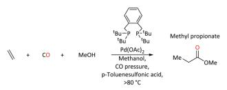
$\begin{tabular}{ll} Scheme 1 & Synthesis of methyl propanoate at Pd(P,P) catalyst with DTBPX ligand system. \end{tabular}$
