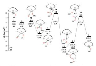
Scheme 3 Carbomethoxy pathway **A**: free-energy profile [kcal  $mol^{-1}$ ] relative to Pd-OMe complex 1 with calculations carried out at the B3PW91-D3/ECP2/PCM//B3PW91/ECP1 level of theory using methanol as the model solvent, and terminating at protonolysis with an overall barrier of 32.9 kcal mol<sup>-1</sup>. Final free energies  $\Delta G$  and enthalpies ( $\Delta H$ ).
