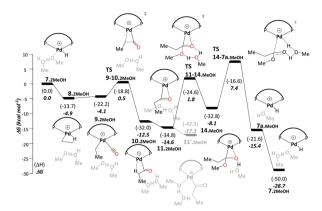
Scheme 5 Hydride-hydroxyalkylpalladium pathway C: free energy profile using methanol as the model solvent at the B3PW91-D3/ECP2/PCM level. Energies are in kcal mol<sup>-1</sup> relative to **7.2MeOH**. Explicit solvent molecules are shown in light grey colour. Final free energies  $\Delta G$  and enthalpies ( $\Delta H$ ).
