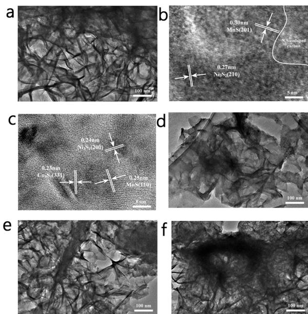
Fig. 4 (a) TEM image of NCMS<sub>x-10</sub>; (b and c) HRTEM images of NCMS<sub>x-10</sub>; (d) TEM image of NCMS<sub>x-5</sub>; (e) TEM image of NCMS<sub>x-15</sub>; and (f) TEM image of NCMS<sub>x-20</sub>.
