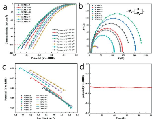
Fig. 5 (a) HER polarization curves (iR-corrected) obtained at a scan rate of 2 mV s<sup>-1</sup>; (b) HER electrical impedance maps; (c) the Tafel slopes of the materials; and (d) results of the 100 h chronopotentiometry test of NCMS<sub>x</sub> under HER.
