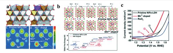
Fig. 7 Activating the basal plane of LDH for water oxidation.<sup>66</sup> (a) Schematic structure and electron density evolution based on DFT calculations, (b) four-electron mechanism of the oxygen evolution reaction and Gibbs free energy evolution based on DFT calculations, and (c) cyclic voltammetry (CV) of different catalysts for the OER tested.
