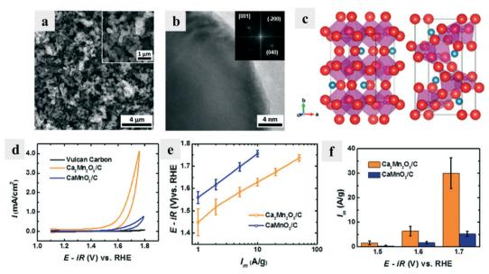
Fig. 8 Oxygen-deficient perovskite  $Ca_2Mn_2O_5$  for the OER. <sup>73</sup> (a) SEM and (b) HRTEM and FFT (inset) images of  $Ca_2Mn_2O_5$ ; (c) unit cell structures of  $CaMnO_3$  (left) and  $Ca_2Mn_2O_5$  (right); (d) iR-corrected data of  $Ca_2Mn_2O_5/C$ ,  $CaMnO_3/C$ , and Vulcan carbon XC-72; (e) Tafel plot of mass activities; (f) mass activities at various applied potentials.
