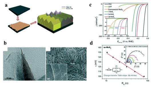
Fig. 6 Effects of high index faces on the catalytic performance of MoS<sub>2</sub>.<sup>54</sup> (a) Schematic illustration of stepped edge surface-terminated MoS<sub>2</sub> arrays (se-MoS<sub>2</sub>), (b) HRTEM image of the se-MoS<sub>2</sub> layers showing that the crystal fringes of the S-Mo-S layers along the edge are stepped, (c) polarization curves and (d) charge-transfer Tafel plots of se-MoS<sub>2</sub> and control catalysts.
