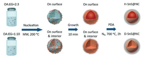
Scheme 1 Schematic illustration of the experimental procedure and proposed formation mechanism for the hollow (top) and dense (bottom) SnS submicrospheres composed of self-assembled nanosheets embedded in a nitrogen-doped carbon shell.
