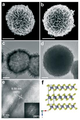
Fig. 3 SEM and TEM images of H- and D-SnS<sub>2</sub>: (a and c) H-SnS<sub>2</sub>, (b and d) D-SnS<sub>2</sub>. (e) HRTEM image of the cross-section of the nanosheets in H-SnS<sub>2</sub> and fast Fourier transform pattern (inset). (f) Crystal structure of hexagonal SnS<sub>2</sub> along the b axis. Scale bars in a)-d) are 200 nm.
