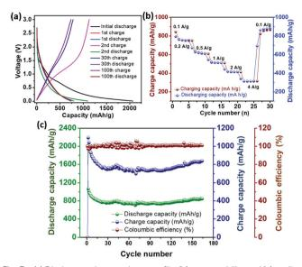
Fig. 3 (a) Discharge-charge voltage profile, (b) rate capability and (c) cycling performance of the electrode containing 3 in the half-cell w. r. t. Li/Li+.
