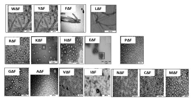
Fig. 7 TEM images showing the self-assembly of dipeptides containing a conformation-restricted residue,  $\alpha, \beta$ -dehydrophenylalanine at their C-terminal. Formation of self-assembled nanostructures by modified dipeptides (X\( \Delta \text{Phe} \)) depending on their X-residue.
