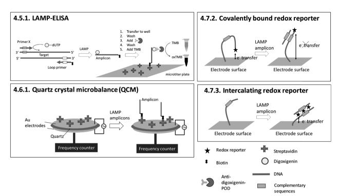
Fig. 9 Schematic illustrations of 4.5.1. LAMP-ELISA, <sup>151</sup> 4.6.1. quartz crystal microbalance (QCM), <sup>153</sup> 4.7.2. covalently bound redox reporter <sup>158</sup> and 4.7.3. intercalating redox reporter <sup>159</sup> (redrawn according to the references).
