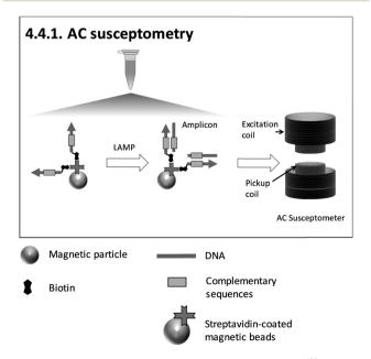
Fig. 8 Schematic illustration of 4.4.1. AC susceptometry<sup>150</sup> (redrawn according to the references).
