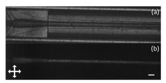
Fig. 5 Jetting of a core of RO-TN 651 within a sheath of 12.5% PI in n-hexane and a coagulation bath of 7% LiBr and 10% PVP in ethanol, as viewed between (a) uncrossed polarisers and (b) crossed polarisers. The birefringent jet in (b) comes from the jetting of the RO-TN. Scale bar 200  $\mu m$ . Flow rates are 1.25 mL  $h^{-1}$  bath, 0.45 mL  $h^{-1}$  polymer, and 0.60 mL  $h^{-1}$  liquid
