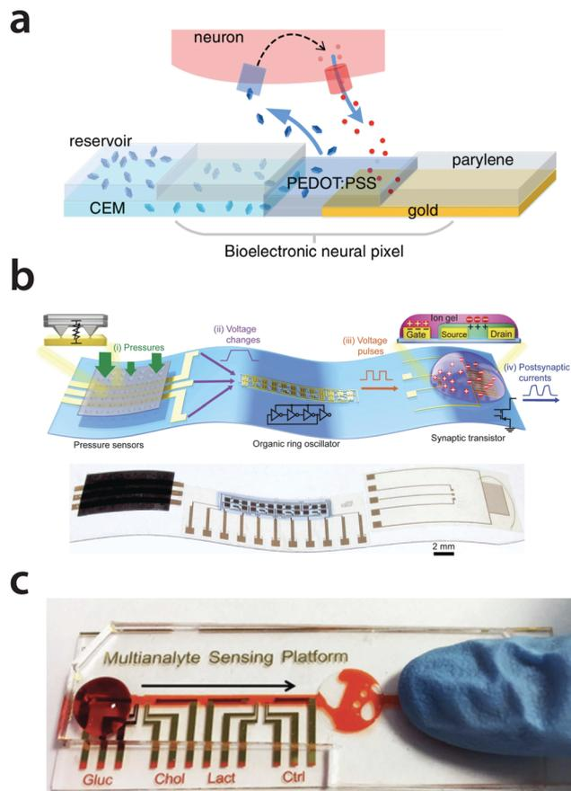
Fig. 3 Examples of transducing, sensing and actuation microsystems. (a) Bioelectronic neural pixel with chemical stimulation and electrical sensing at the same site.<sup>33</sup> (b) Bioinspired flexible organic artificial afferent nerve.<sup>34</sup> (c) Organic-transistor array-based multi-analyte sensing platform for saliva testing.<sup>35</sup>
