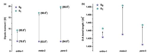
Fig. 5 Changes in the dipole moment and (bracketed) D-A bond angles (a) and D-A bond lengths (b) of DMAC-BZN isomers in ground and excited states (rBMK/6-31G(d) on X-ray geometries for  $S_0$  and TDA-DFT BMK/6-31G(d) for  $S_1$ ).
