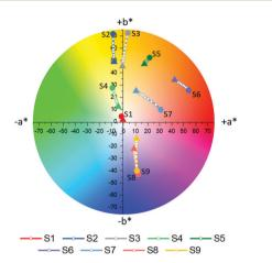
Fig. 4 Color tracks obtained for S1-S9 when titrating against Na+  $(Na^{+} = 0 \text{ mM} \text{ denoted by filled circle}, Na^{+} = 6.66 \text{ mM} \text{ denoted by filled}$ triangle, with increments of 0.66 mM noted by white filled circles).
