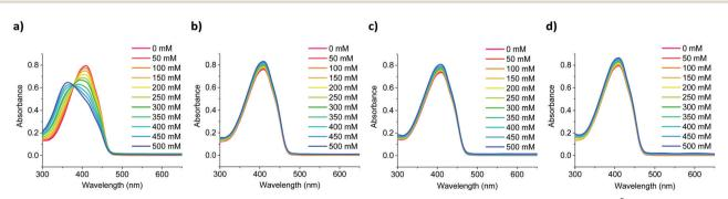
Fig. 3 Representative UV-Vis absorption spectra of **S4** in a 1:3 mixture of water: tetrahydrofuran (**S4** concentration  $4 \times 10^{-5}$  M) upon incrementing (a)  $Na^+$ , (b)  $Li^+$ , (c)  $K^+$  and (d)  $Ca^{2+}$  concentrations (0–500 mM).
