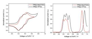
Fig. 2 Cyclic voltammograms (CV) (left) and square wave voltammetry (SWV) of TPB(2-MeOTAD) and TPB(2-TPTZ) in DCM solution with supporting electrolyte 0.3 M tetrabutylammonium hexafluorophosphate referenced to ferrocene
