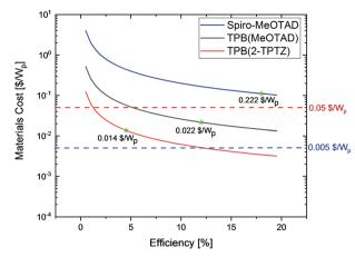
Fig. 6 Calculated material cost-per-peak-Watt (\$ per W<sub>p</sub>) as a function of solar cell efficiency. The star marks indicate device efficiencies delivered in this work
