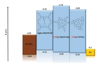
Energy level diagram and device architecture of perovskite solar Fig. 4
