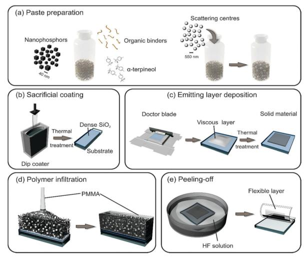
Fig. 1 Description of the different steps of preparation and fabrication of a flexible photoluminescent nanophosphor-based material with and without the inclusion of scattering centres from an initial dispersion of nanophosphors.
