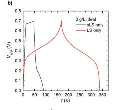
Fig. 5 Simulated electrode response under galvanostatic charge—discharge at 1689  $\mu$ A (2 A g<sup>-1</sup>) for 1\_2 electrodes. (a) At steady operation (after long cycling), and (b) for idealized cases where LS is confined in electrode domain in only solid (sLS) or dissolved (LS) form.
