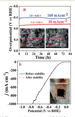
Fig. 8 (a) Chronopotentiometric curve of Cuf@Ni<sub>5</sub>P<sub>4</sub> at a current density of 10 and 160 mA cm $^{-2}$ , inset shows the SEM images obtained before and after the test. (b) LSV of Cuf@Ni<sub>5</sub>P<sub>4</sub> before and after the chronopotentiometric test.
