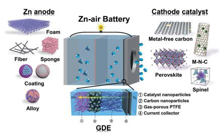
Fig. 1 Schematic configuration of Zn-air batteries including the GDE structure, different candidate materials for cathode electrocatalysts and different forms of Zn anode materials.
