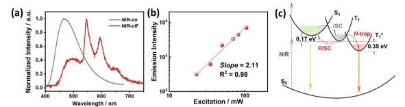
Fig. 5 (a) Two-photon-induced steady-state emission and delayed emission (delay = 8 ms) of o-Cz excited with a 808 nm femtosecond laser; (b) plots of emission intensity varying with input laser density (collected at 542 nm); (c) proposed mechanism of the two-photon induced ultralong phosphorescence in o-Cz. The energy levels are obtained with experimental spectra of the crystalline o-Cz.
