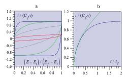
Fig. 13 Variation of the dimensionless current function with (a) the dimensionless potential,  $(E-E_i)/(E_f-E_i)$  for several values of the parameter  $t_f/t_v=0.1$  (blue), 0.5 (green), 2 (grey), and 20 (red), with negligible solution resistance  $R_u=0$ ; (b) with the dimensionless time  $t/t_f$ , with  $t_f/t_v=0.5$  and  $R_u=0$  (blue line). The green line is the limiting behaviour observed at short times.
