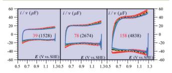
Fig. 6 Cyclic voltammetry current–potential responses at various scan rates ( $\nu$ ) of CoP $_{\rm i}$  films at pH 7 in the presence of 1 mM Pi and 100 mM KNO $_{\rm 3}$ .  $\nu$  (V s $^{-1}$ ): 1 (red), 2 (orange), 3 (black), 4 (green), 5 (cyan), 6 (gray), 7 (magenta), and 8 (blue). The numbers on each diagram are the values of film thickness in nm and, between parentheses, the value of the plateau capacitance in  $\mu F$  cm $^{-2}$ . Adapted from ref. 18, with permission.
