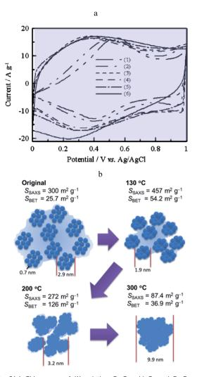
Fig. 10 0(a) CV curves of (1) pristine  $RuO_x \cdot nH_2O$  and  $RuO_x \cdot nH_2O$  annealed in air for 2 h at (2) 150, (3) 200, (5) 350 and (6) 400 °C. CV curves were measured in 0.1 M  $H_2SO_4$  at 25 mV s<sup>-1</sup> from ref. 29 with permission. (b) Schematic diagram of the hierarchical nanostructure in  $RuO_x \cdot nH_2O$  changing with the annealing temperature from ref. 32 with permission.
