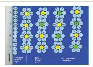
Fig. 11 The electrochemical double layer.
