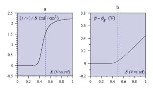
Fig. 9 (a) Forward CV scan for with  $C_{\rm d}=2.55$  mF cm $^{-2}$  (i.e. capacitance of a 40 nm CoP<sub>i</sub> film),  $F^2N/RT=20$  mF cm $^{-2}$  (i.e.  $N=8\times10^{20}$  cm $^{-3}$  for a 40 nm film),  $E^{0,\rm ap}-\Delta E^0/2+\phi_{\rm S}=0.5$  V (dashed vertical line), T=298 K. (b) Evolution of the film inner potential. Adapted from Fig. 5 in ref. 19 with permission.
