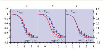
Fig. 14 Variations of the capacitance with scan rate from  $MnO_2$  electrodes in ref. 69 (from multicycle limiting CV responses). (a) Amorphous, (b) birnessite, (c) spinel, in aqueous  $Li_2SO_4$  (red) and  $(NMe_4)_2SO_4$  (blue). Data points: closed circles. Full lines: fitting of data by means of a transmission line model. Dotted lines: simulations with a RC model (see ref. 68 for details).
