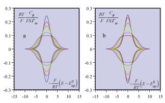
Fig. 4 Formal capacitance  $C_{\phi}$  vs. electrode potential as a function of the parameter  $2(a_{\rm Q}+a_{\rm P}-2a_{\rm PQ})=F\Delta E^0/RT=0.1$  (blue), 1 (red), 2 (green), 3 (yellow), 4 (gray), and 5 (magenta). (a) Calculated from interaction coefficients,  $a_{\rm P}$ ,  $a_{\rm Q}$  and  $a_{\rm PQ}$  linearly varying with the surface concentrations. (b) Calculated from the square standard potential distribution
