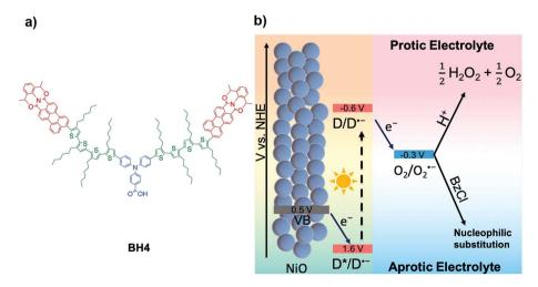
Scheme 1 (a) Molecular structure of BH4. (b) Schematic representation of the DSPEC for H<sub>2</sub>O<sub>2</sub> production in protic electrolyte and nucleophilic substitution in aprotic electrolyte.
