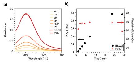
Fig. 2 (a) Absorbance of triiodide (generated from reaction with  $H_2O_2$ ) at different time (0 h, 1 h, 2 h, 3 h, 4.4 h, 7 h, 18.6 h, 24 h). (b) Concentration of  $H_2O_2$  from titrations and corresponding faradaic efficiency during bulk electrolysis with applied bias at 0.42 V vs. RHE under 1 sun light illumination.
