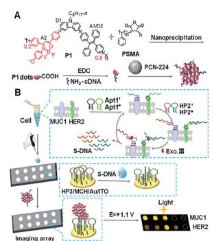
Scheme 1 Schematic diagram of (A) preparation of Pdots@PCN-224 as an ECL probe and (B) ECL imaging array for the analysis of two kinds of membrane proteins with target-mediated cyclic amplification.
