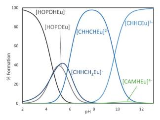
Fig. 6 Speciation diagram for a competition between 3,4,3-LI(1,2-HOPO), 3,4,3-LI(CAM), and 3,4,3-LI(CHHC) abbreviated HOPO (gray), CAM (green), and CHHC (blue), respectively, in the presence of Eu $^{3+}$ . [HOPO] = [CAM] = [CHHC] = [metal] = 25  $\mu$ M, I = 0.1 M, T = 25  $^{\circ}$ C. Only the major species were labeled on the plots for clarity.
