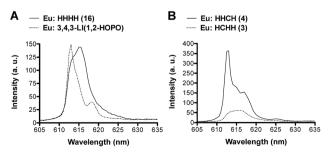
Fig. 5 The  ${}^5D_0 \rightarrow {}^7F_2$  emissive transition of the Eu complexes formed with (A) 3,4,3-LI(1,2-HOPO) (dotted line) and (16) HHHH (solid line); (B) (3) HCHH (dotted line) and (4) HHCH (solid line).
