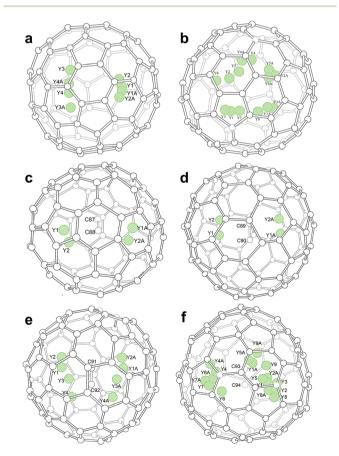
Fig. 1 Perspective drawings showing the internal yttrium sites. (a) 8 in  $Y_2 @ C_s(6) - C_{82}$ , (b) 14 in  $Y_2 @ C_{3v}(8) - C_{82}$ , (c) 4 in  $Y_2 C_2 @ C_s(15) - C_{86}$ , (d) 4 in  $Y_2C_2@C_1(26)-C_{88}$ , (e) 8 in  $Y_2C_2@C_2(41)-C_{90}$ , and (f) 17 in  $Y_2C_2@C_2(61)-C_{90}$
