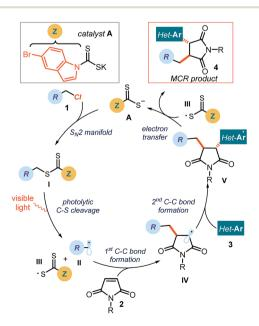
Fig. 2 Proposed mechanism for the visible-light-driven three-component radical reaction; Z: chromophore.
