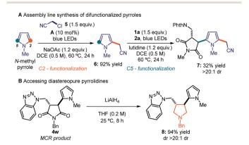
$\begin{tabular}{lll} Scheme 1 & (A) Photochemical radical assembly line and (B) derivativation of MCR products. \end{tabular}$
