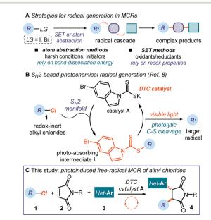
Fig. 1 (A) Classical radical-generating strategies to initiate multi-component reactions require precursors with suitable bond-dissociation energies (BDE) or redox properties. (B) Our recently developed  $S_{\rm N}2$ -based method to photochemically generate radicals is not reliant on the redox properties of substrates. (C) Proposed photoinduced three-component radical reaction using redox-inert alkyl chlorides 1, mediated by dithiocarbamate (DTC) anion catalysis.
