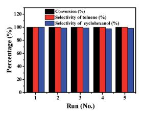
Fig. 9 Catalytic cycling tests of Ni/Al<sub>2</sub>O<sub>3</sub>-600 catalyst during the hydrogenation of benzyl phenyl ether. Reaction conditions: benzyl phenyl ether ( $\alpha$ -O-4) (185 mg, 1 mmol), Ni/Al<sub>2</sub>O<sub>3</sub>-600 (20 mg), solvent (10 mL), 150 °C, stirring at 1000 rpm, 5 h.
