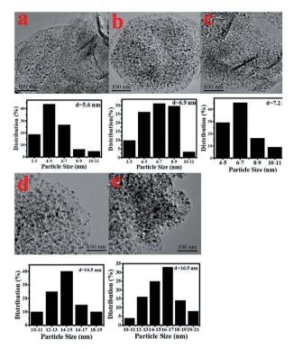
Fig. 3 TEM images of the as-prepared Ni/Al $_2$ O $_3$ -T catalysts and particle size distribution of the Ni nanoparticles ((a) Ni/Al $_2$ O $_3$ -500; (b) Ni/Al $_2$ O $_3$ -550; (c) Ni/Al $_2$ O $_3$ -600; (d) Ni/Al $_2$ O $_3$ -650; (e) Ni/Al $_2$ O $_3$ -700).
