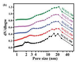
Fig. 2 (a)  $\rm N_2$  adsorption/desorption isotherms of Ni/Al $_2\rm O_3$ - $^T$  catalyst and, (b) corresponding Barrett-Joyner-Halenda (BJH) pore-size distribution curve.
