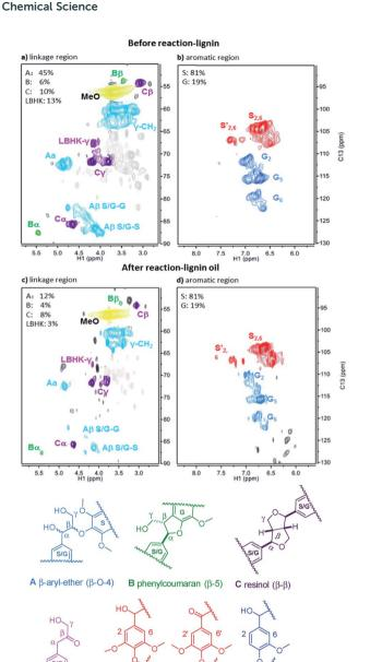
Fig. 8 2D HSQC NMR spectra of beech lignin in DMSO- $d_6$  before reaction (a and b); and lignin oil after reaction (c and d). Note: the percentage of linkages A, B, C and LBHK was calculated based on per 100 C9 unit, see Fig. S4† for the detailed integration process.
