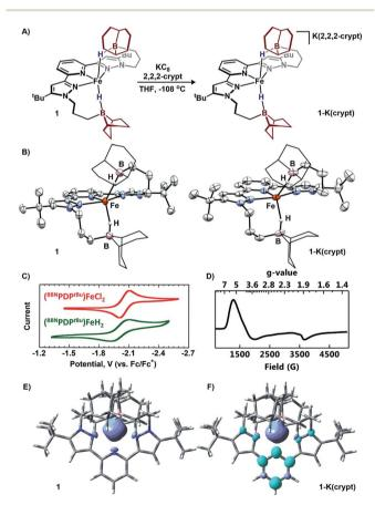
Fig. 3 (A) Reduction of 1. (B) Molecular structures of 1 and 1-K(crypt) (50% probability ellipsoids). For clarity, the 9-BBN substituents are displayed in wireframe. (C) Electrochemical comparison between 1 and ( $^{\rm BBN}$ PDP $^{\rm tBu}$ )FeCl $_2$ . (D) X-band EPR of 1-K(crypt) at 10 K in 1:1 toluene/THF. (E and F) Spin-density isosurface plots (0.002 a.u.) of 1 and 1-K(crypt), respectively.
