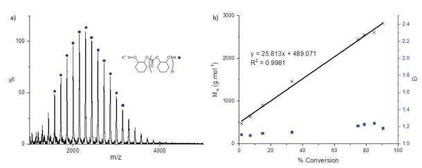
Fig. 3 (a) MALDI-ToF mass spectrum of poly(cyclohexene carbonate) formed from catalyst 2c (0.1 mol%) with 10 equivalents of added CHD. (b) Plot of the polycarbonate  $M_n$  (black crosses) and D (blue squares) versus % CHO conversion. Reaction conditions: 2b/CHO/CHD = 1/1000/10, 80 °C, 5 M in toluene (Fig. S65–S72†).
