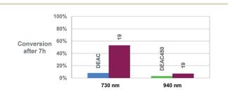
Fig. 6 Comparative histogram showing the conversion of the uncaging reaction (Gly release) after 7 h of two-photon irradiation at 730 and 940 nm in similar conditions (1.2 mL, 1 W).
