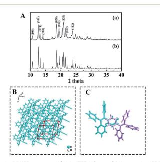
Fig. 2 (A) XRD patterns of (a) the TPE NCs and (b) the standard PDF card of the TPE crystal, (B) the predicted morphology of TPE crystals, and (C) the predicted interaction between the two TPE molecules represented in different colors.
