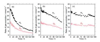
Fig. 1 Time courses of water-splitting activity of SrTiO<sub>3</sub>:Al loaded with (a) RhCrO<sub>x</sub>, (b) RhCrO<sub>x</sub> and 0.3 wt% Co species, and (c) RhCrO<sub>x</sub>, 0.3 wt% Co species and 3 wt% TiO2. Reaction conditions: photocatalyst, 0.5 g; reaction solution, 370 mL distilled water; reaction temperature, 291 K; light source, 450 W high-pressure Hg lamp ( $\lambda$  > 300 nm).
