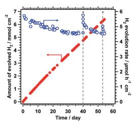
Fig. 4 Time course of water splitting activity of  $5 \times 5 \text{ cm}^2 \text{ TiO}_2/\text{CoOOH/RhCrO}_x/\text{SrTiO}_3$ :Al sheet in panel reactor. Reaction conditions: photocatalyst, 20 mg; reaction solution, 1 mm deep distilled water; reaction temperature, 291 K; light source, AM 1.5G solar simulator. Asterisk symbols (\*) indicate interruption of the illumination for two days.
